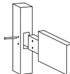
•Tenons are a key element of construction. A board's end is cut off for insertion into a mortise. Tenons are then secured with wood pins.
