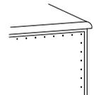
•Case backs (1/4" thick) with recessed back panels.
