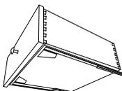
•Drawers suspended with heavy duty undermount **full extension soft-close** guides allowing for effortless opening and closing.
